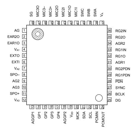
**48-Pin Plastic TQFP**
