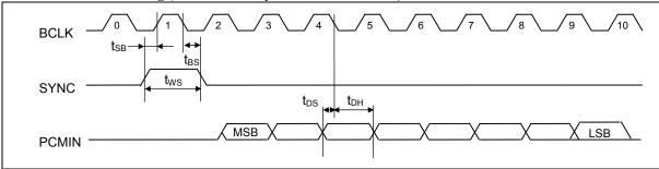
Figure 6 PCM Interface Timing
