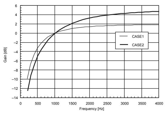
Figure 8 Slope Filter Frequency Characteristics
