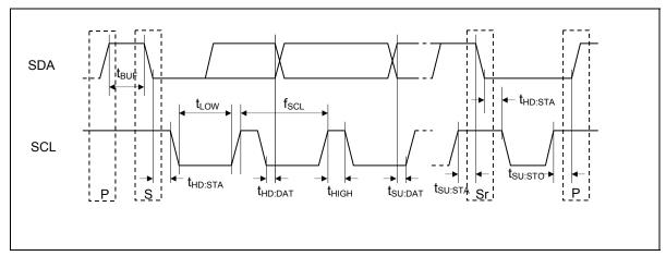
Figure 7 I<sup>2</sup>C Interface Timing
