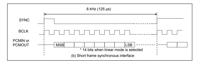
Figure 2 PCM Interface Basic Timing Diagram
